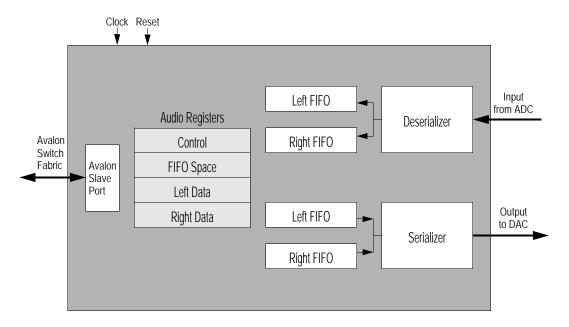
Figure 1. Block Diagram for Audio Core
